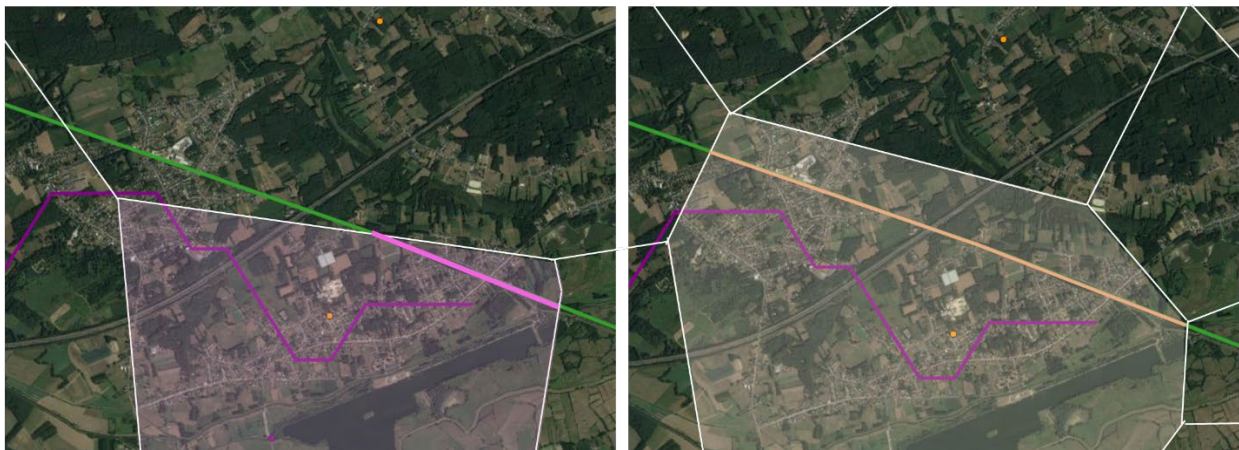
Figure 20: Railway segment assignment (based on Voronoi polygons) to define dependencies between railway, telecom and electricity networks
